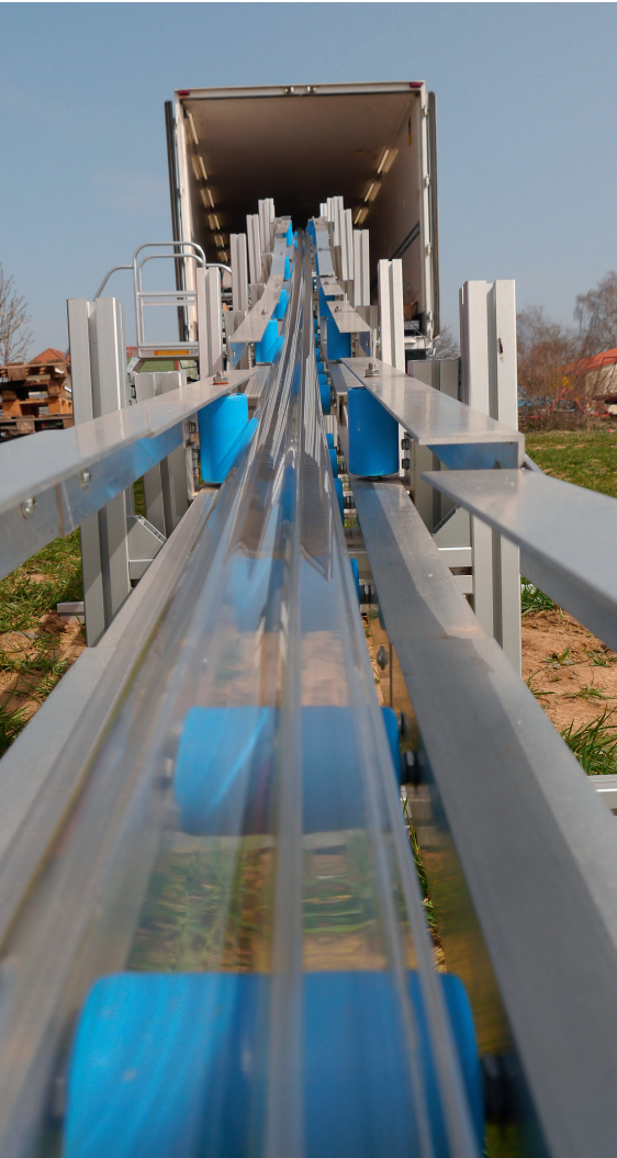
Fig. 2. The company Algoliner has developed a mobile PMMA extrusion line that enables resource-saving photobioreactors to be installed at almost any location. © Algoliner
